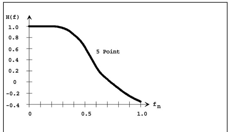
**Figure 7. Transfer Function for Unequally Weighted Averages**
