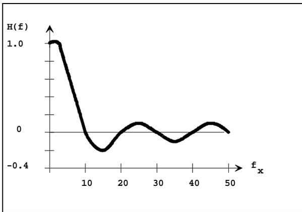
**11-Point Equally Weighted Sample,  $f_s = 110$  Hz**
