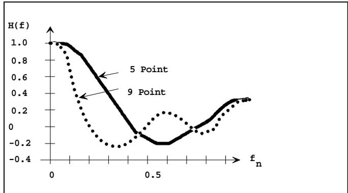
**Figure 6. Transfer Function for Equally Weighted Running Averages**
